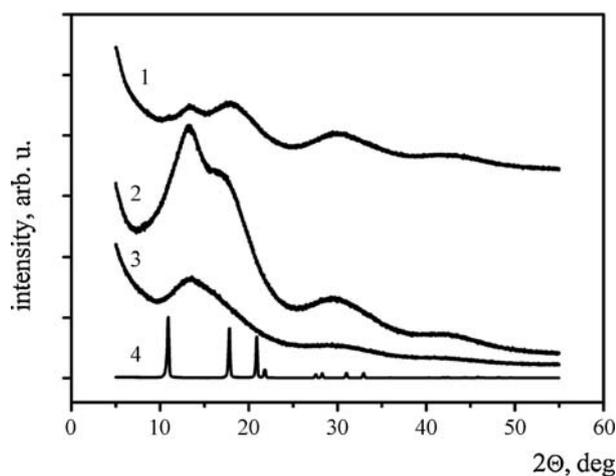
**Figure 5.** WAXD spectra of neat a-PMMA (1), a-PMMA- $C_{60}$  SD composite (2), a-PMMA- $C_{60}$  RD composite (3) and fullerene  $C_{60}$  powder (4) used in the work. According to TGA data the volume content of toluene in the polymer samples is  $\sim 8\%$ .
