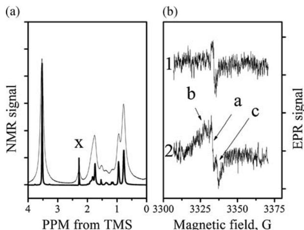
**Figure 3.** (a) <sup>1</sup>H NMR spectra of PMMA-C<sub>60</sub> (thick line) and PMMA-MWNT (thin line) composites dissolved in deuterated chloroform. Cross sign X denotes NMR signal of residual toluene. (b) EPR spectra taken at room temperature for PMMA-C<sub>60</sub> composite before (curve 1) and after (curve 2) heat treatment at  $\sim 170^\circ\text{C}$  in dynamic vacuum of  $\sim 4\text{ mbar}$ .
